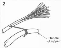
Extract the rip cord and wrap it around a suitable bar (eg handle of nippers). Pull slowly to split the cable sheath to the required length.
