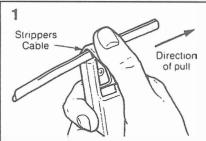
Using correctly adjusted Strippers Cable Sheath 7. make two diametrically opposite longitudinal cuts on the cable sheath to expose 150-200mm of cable core.
