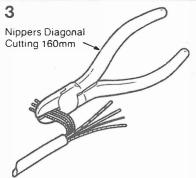
Remove excess sheath and cut strength members to a length of 20mm.
