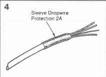
Fold back strength members along sheath and place a Sleeve Dropwire Protection 2A over the strength members and sheath.
