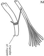
required length. Pull slowly to split the cable sheath to the suitable bar (eg handle of nippers). Extract the rip cord and wrap it around a
