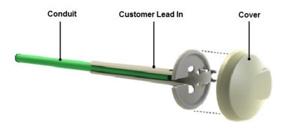
It can accommodate either 1 x 5mm OD fibre cable or up to 2 x 4.8mm OD unsheathed fibre cables with a 15mm Bend Radius.
